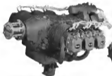
Above is the recently announced Franklin six-cylinder Model 8-110-73 engine at the latest design. The engine develops 120 hp. at 1500 r.p.m.
